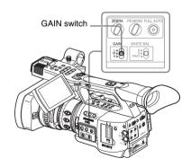
The gain value at each of the switch positions are set at the factory are as follows:
